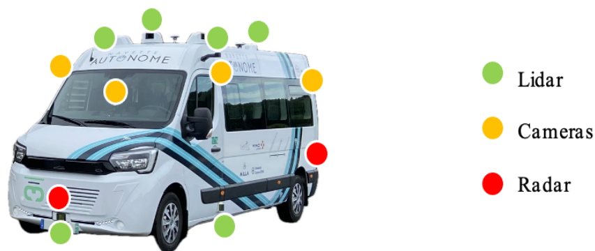
Figure 3. – Sensor Distribution and Perception System on the MOBAUTO 2 Shuttles
